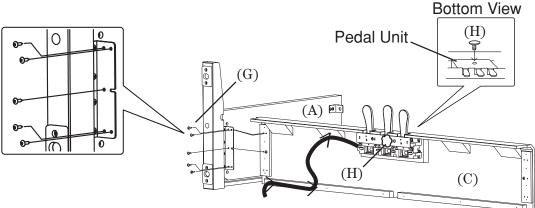
**1.** Insert the Adjuster (H) on the Pedal Unit.
